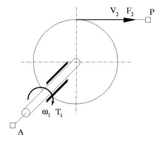
The wheel and the axle have the same axis, and the axis is assumed to be rigidly connected to the frame, thus making this mechanism an ideal converter of mechanical
