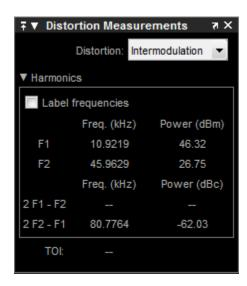
The intermodulation distortion measurement automatically locates the fundamental, first-order frequencies (F1 and F2). It then computes the frequencies of the third-order intermodulation products (2\*F1-F2 and 2\*F2-F1).
