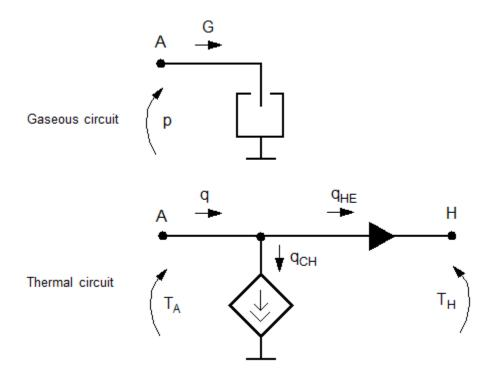
The diagram shows that the heat flow  $\boldsymbol{q}$  to the chamber consists of two components:
