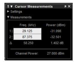
The **Cursor Measurements** panel appears as follows for spectrograms.
