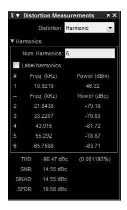
The harmonic distortion measurement automatically locates the largest sinusoidal component (fundamental signal frequency). It then computes the harmonic frequencies and power in each harmonic in your signal. Any DC component is ignored. Any
