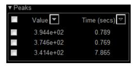
The numerical values displayed in the **Value** column are equivalent to the **pks** output argument returned when you run the **findpeaks** function. The numerical values displayed in the second column are similar to the **locs** output argument returned when you run the **findpeaks** function.
