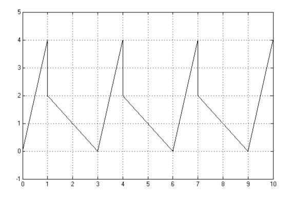
The signal starts at 0 and consists of two linear segments. The duration of the first segment is 1 second, the segment starts at 0 and ends at 4. The signal is discontinuous, and the end value of the first segment is different than the start value of the second segment, therefore they are connected by a vertical line. The second segment starts at 2, lasts for 2 seconds, and ends at 0, after which the sequence repeats.
