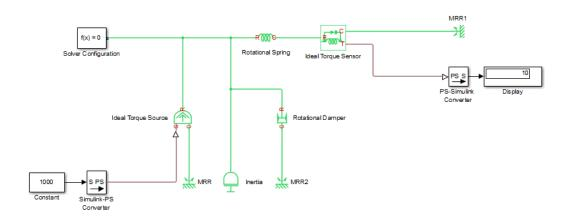
**Note** Currently, physical units are not propagated through the blocks in the Physical Signals library, such as PS Add, PS Gain, and so on. If your diagram contains a Physical Signals block after a Simulink-PS Converter block, the unit specification in the Simulink-PS Converter block does not propagate to the rest of the network.
