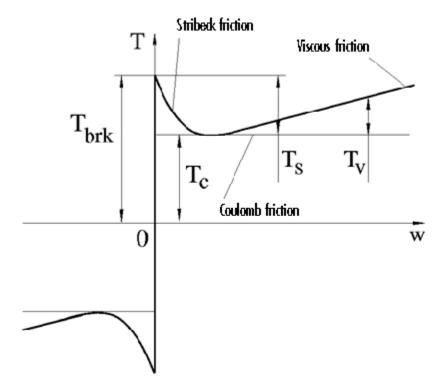
The Stribeck friction,  $T_S$ , is the negatively sloped characteristics taking place at low velocities (see [1]). The Coulomb friction,  $T_C$ , results in a constant torque at any velocity. The viscous friction,  $T_V$ , opposes motion with the torque directly proportional to the relative velocity. The sum of the Coulomb and Stribeck frictions at the vicinity of zero velocity is often referred to as the breakaway friction,  $T_{brk}$ . The friction is approximated with the following equations:
